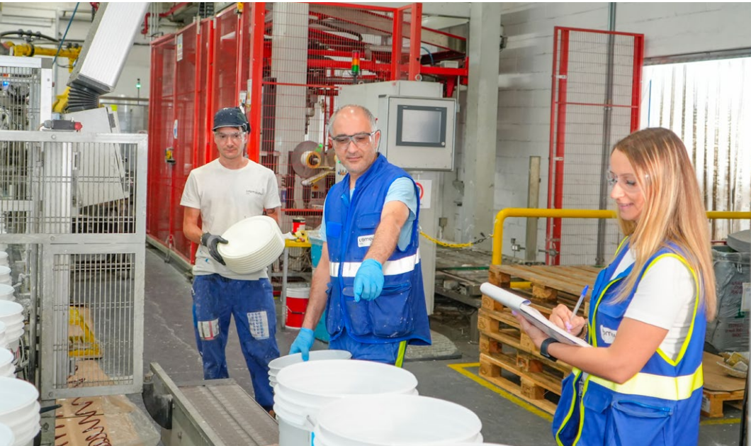
Preparation of buckets and lids for future paint cans on a packaging line.
